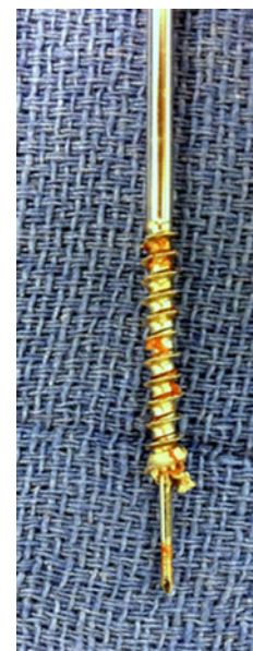
Fig. 1 Intraoperative anteroposterior fluoroscopic image showing the unraveled Synthes 4.0 mm cannulated screw over the guide wire
